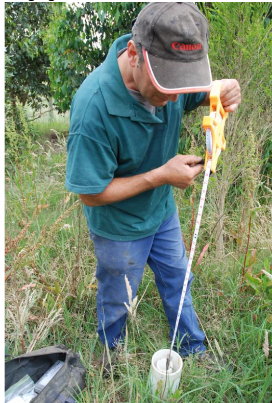
Rocky measuring ground water table depth
